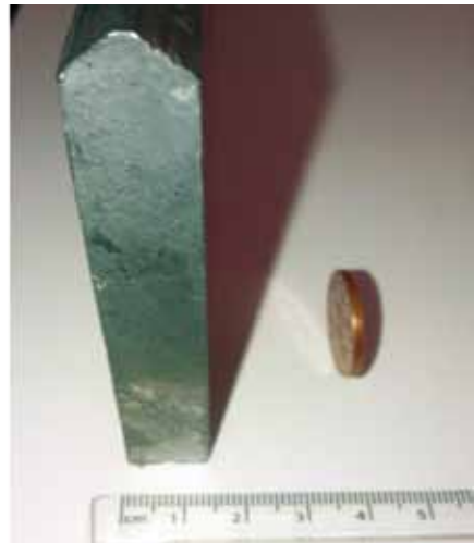
Figure 12: A 15-mm lead brick; such bricks help to provide additional shielding
